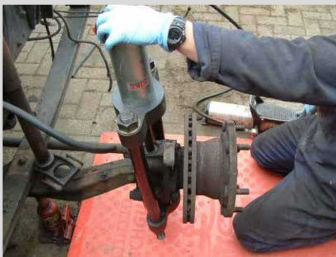
Replacing a sized king pin can be a time consuming process. Using the KPP20 means keeping trouble and labour time for this kind of job to a minimum.
